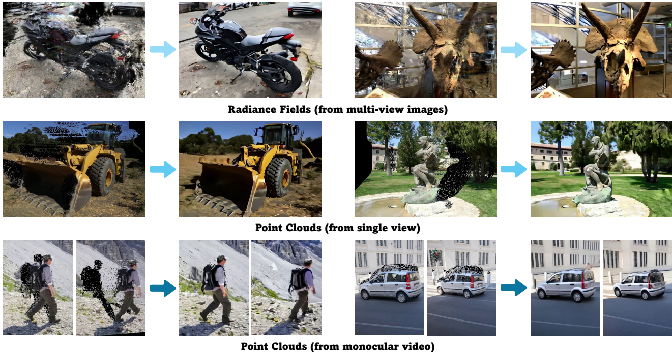
Figure 1. We introduce ViewExtrapolator , a novel approach that leverages the generative priors of Stable Video Diffusion for novel view extrapolation, where the novel views lie far beyond the range of the training views. ViewExtrapolator effectively refines the artifact-prone renderings (left side of arrows) of radiance fields or point clouds, to more realistic renderings with fewer artifacts (right side of arrows).
