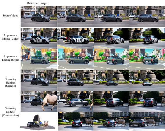
Figure 5. Applications. Top : Appearance editing—a single edited reference frame (e.g., zebra pattern or anime style) is propagated consistently across all novel viewpoints via our foreground-complete proxy. Bottom : Geometry editing—manipulating the point cloud (scaling or compositing) produces plausible redirected videos from modified 4D geometry.
