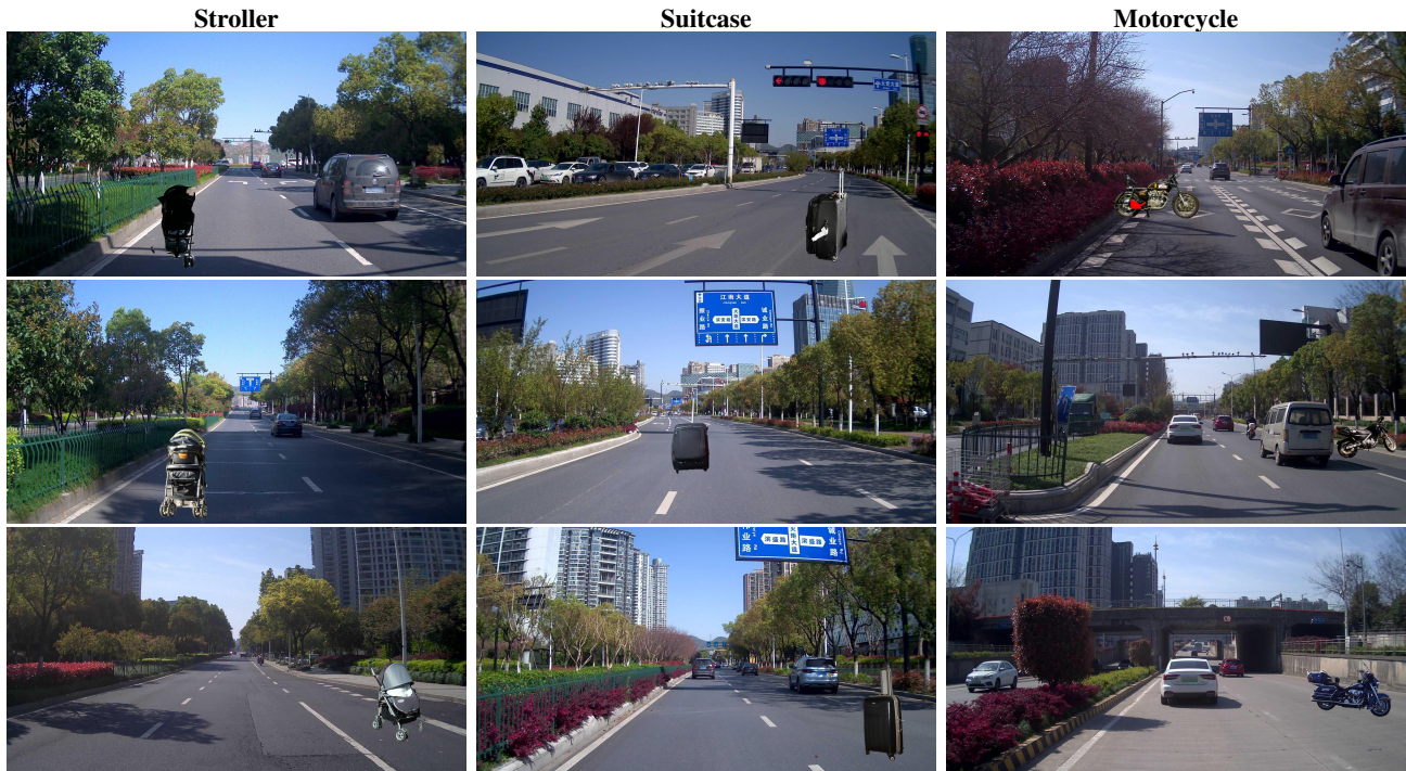
Figure 6. Synthetic training images generated using the CopyPaste baseline. Object instances from the LVIS dataset are composited into ONCE driving scenes using alpha blending within predefined bounding boxes. Because pasted instances are taken directly from existing images, they may exhibit artifacts originating from the source dataset, such as incomplete objects due to occlusion in the original image, fragmented or noisy segmentation masks, and inconsistencies in lighting, texture, or shadows relative to the target scene. Each column corresponds to one target category (stroller, suitcase, and motorcycle).
