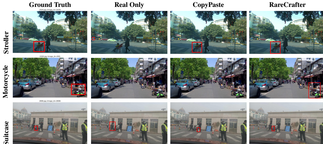
Figure 2. Qualitative object detection results on the CODA2022 dataset. The detection models are trained under three regimes: real-only data, real data augmented with CopyPaste, and real data augmented with RareCrafter. In the first row, the detector trained on real-only data incorrectly localizes another object as a stroller. In the second row, both the real-only and CopyPaste models fail to detect the motorcycle. In the third row, the real-only model confuses a pedestrian carrying a suitcase with the suitcase itself, while CopyPaste incorrectly localizes another object as a suitcase. In contrast, RareCrafter correctly detects the suitcase without misclassifying the pedestrian.
