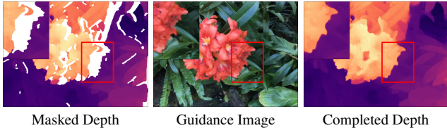
Figure 4. The depth completion model takes a masked depth along with a guidance image as input and completes the depth in the masked region using the guidance of the RGB image.
