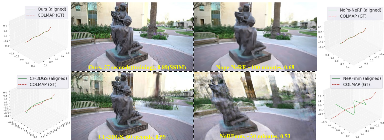
Figure 1. Novel View Synthesis Comparisons (Sparse-View, Pose-Free) . We introduce InstantSplat, an efficient framework for simultaneous pose estimation and novel view synthesis in unrestricted scenarios. This approach incorporates 3D priors derived from a dense stereo model, a streamlined framework capable of reconstructing 3D scenes and enabling view synthesis within one minute, for large-scale scenes. Moreover, our method markedly enhances both pose estimation accuracy and rendering quality.
