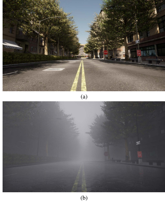
Figure 12. (a) Base weather image rendered using CARLA simulator on top of Unreal 5 engine. (b) Text-2-graphics program synthesis given the prompt "Always have storm weather with 100% cloudy and 100% rainy."
