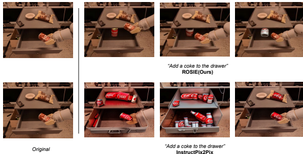
Figure 2. Our augmentation scheme generates more targeted and physically realistic augmentations that are useful for learning downstream tasks, while other text-to-image generation methods such as InstructPix2Pix [5] often makes global changes rendering the image unusable for training.
