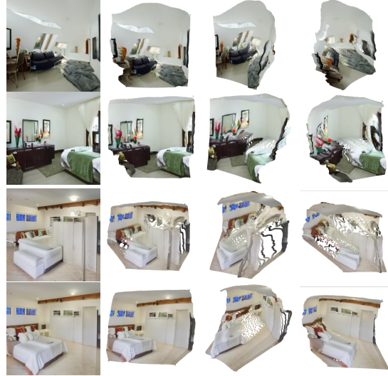
Figure 5. Visualization of point cloud representation obtained by depth information. We compare the results generated from the baseline without (odd rows) and with (even rows) our guidance by showing images and transforming them into point cloud visualizations in four different views.
